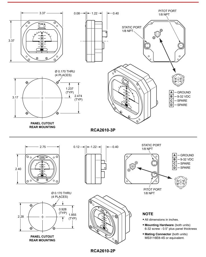
Figure 1, General Dimensions of the RCA2610-P3 and RCA2610-P2
